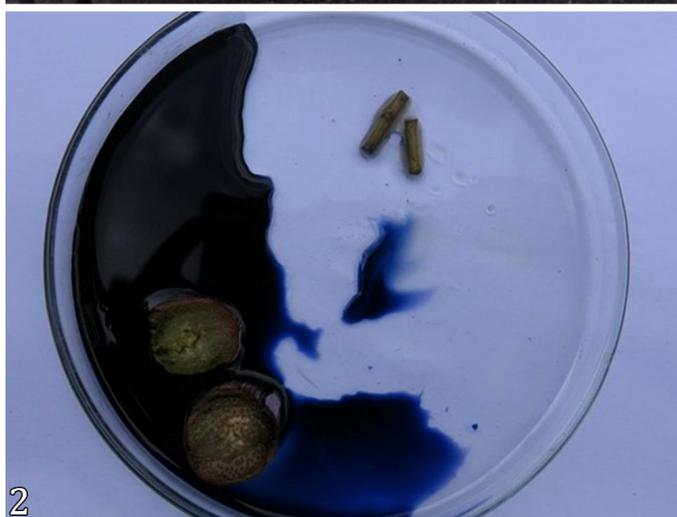
Fig.1-2. (1) LAQUAtwin HORIBA B-743 portable nitrate meter. (2) Diphenylamine test with positive reaction.
