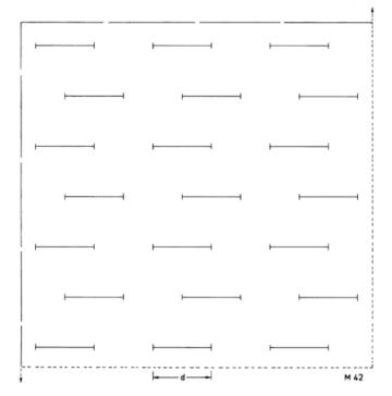
Fig.1.Diagram of the M42 testing system incorporating the forbidden line (dotted line). The elements intercepted by that line should not be considered to avoid the bias of over estimation (Gundersen 1977).
